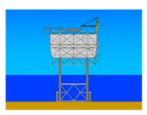
AC/DC Converter Platform of the Wind Farm Field in 40 m water depth weighting 12.000 tons - Basic Design of Topside and Jacket
