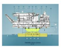
N° 3 Topsides to be installed by Float-over Mating System - Weights ranging of 2.000 5.000 and 10.000 tons Analysis and Design of the Mating system
